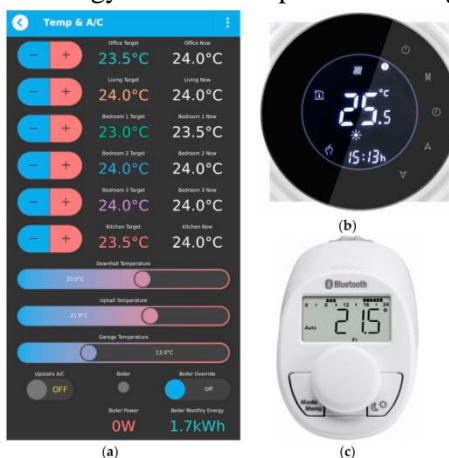
Fig.10 Controlling indoor temperatures with qToggle app (a) together with smart thermostats (b,c).
