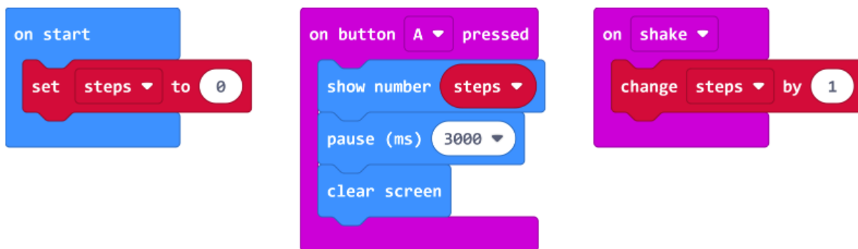
Figure 3. Code in Micro Bit for steps counter
