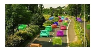
**Mask R-CNN:** This is an extension of Faster R-CNN that can perform both object detection and segmentation. It can be used to segment the license plate from the background and detect the characters onthe plate.
