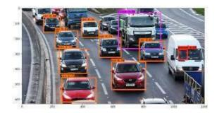
Earlier detection frameworks, looked at different parts of the image multiple times at different scales and repurposed image classification technique to detect objects. This approach is slow and inefficient.YOLO takes entirely different approach. It looks at the entire image only once and goes through the network once and detects
